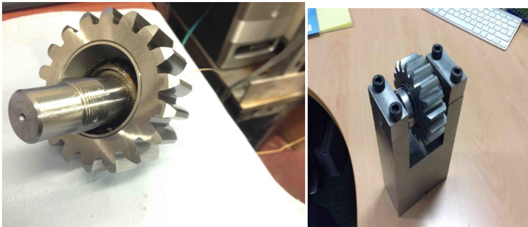
Figure 5 Idler gear and bearing assembly
