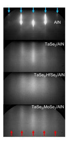
**Figure 2.** (a) RHEED diffraction patterns of the 4 ML MBE-deposited TaSe<sub>2</sub> films on different templates (AlN, HfSe<sub>2</sub> and MoSe<sub>2</sub>) obtained along the  $[1\overline{10}]$  azimuth of the bare AlN(0001) surface, showing good quality epitaxial growth with excellent alignment of the 2D metal with the substrate. Blue and red arrows indicate the diffraction streaks of AlN(0001) and TaSe<sub>2</sub> superstructures, respectively.
