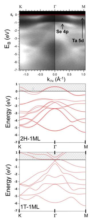
**Figure 3.** Band structure imaging by *in-situ* ARPES of 4 ML-TaSe<sub>2</sub>/AlN (top) and DFT bandstructure calculations for 2H (middle) and 1T (bottom) TaSe<sub>2</sub> phases. Experimental data agree well with the formation of the trigonal prismatic 2H-TaSe<sub>2</sub> phase.
