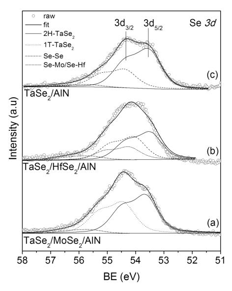
**Figure 5.** Deconvolution of the Se 3d doublets of the 4-ML thin TaSe<sub>2</sub> films grown epitaxially on (a) MoSe<sub>2</sub>, (b) HfSe<sub>2</sub> and (c) AlN templates, showing the formation of a pure (a)/dominant (b) and (c) 2H-TaSe<sub>2</sub> phase in all cases.
