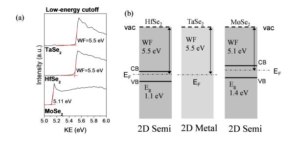
**Figure 6.** (a) Low energy cut off for TaSe<sub>2</sub>, HfSe<sub>2</sub> and MoSe<sub>2</sub> samples, as determined from UPS measurements, (b) Schematic of the HfSe<sub>2</sub>/TaSe<sub>2</sub> and MoSe<sub>2</sub>/TaSe<sub>2</sub> band alignments as derived from UPS measurements, showing workfunction matching according to the electron affinity rule.
