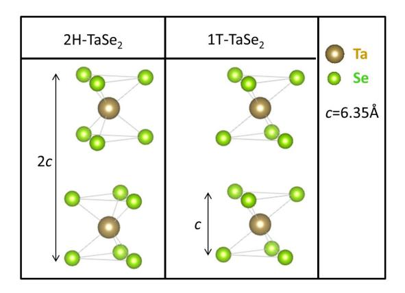
**Figure 1.** The crystallographic structure of the two most common 2H and 1T-TaSe<sub>2</sub> polytypes. The Se-Ta-Se coordination is trigonal prismatic in the 2H structure and octahedral in the 1T structure.
