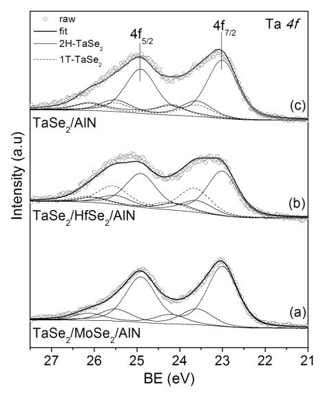
**Figure 4.** Deconvolution of the Ta 4f doublets of the 4-ML thin TaSe<sub>2</sub> films grown epitaxially on (a) MoSe<sub>2</sub>, (b) HfSe<sub>2</sub> and (c) AlN templates, showing the formation of a pure (a)/dominant (b) and (c) 2H-TaSe<sub>2</sub> phase in all cases.
