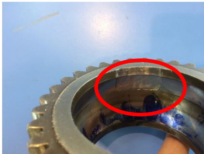
262 Figure 3 Slot across the bearing outer race
