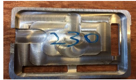
(b) Machined component under an abnormal condition
