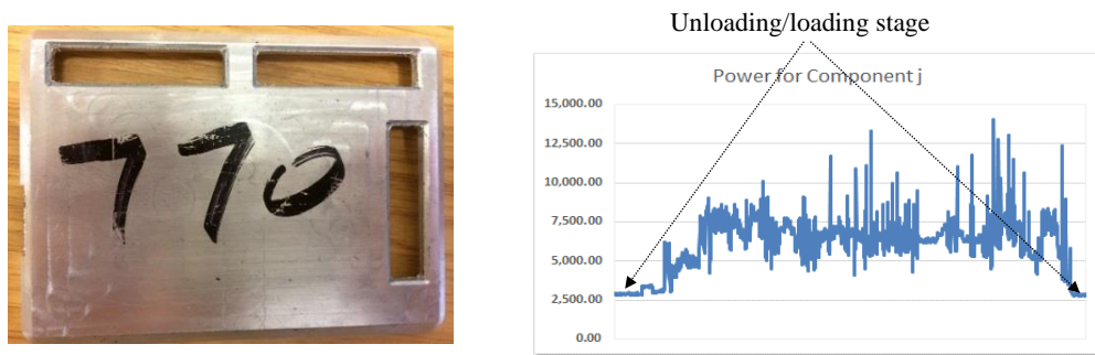
Figure 8: Energy consumption monitored during the unloading/loading stages.
