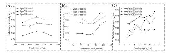
Fig. 4 Effects of grinding parameters on surface roughness: (a) spindle speed (b)worktable feed rate (c)grinding depth on surface roughness
