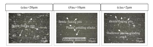
Fig. 5. Grinding surface topography under different grinding depth
