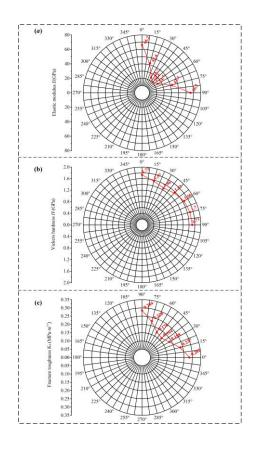
Fig. 2 Directional variations of (a) Elastic modulus, (b) Micro Vikers hardness and (c) Fracture toughness
