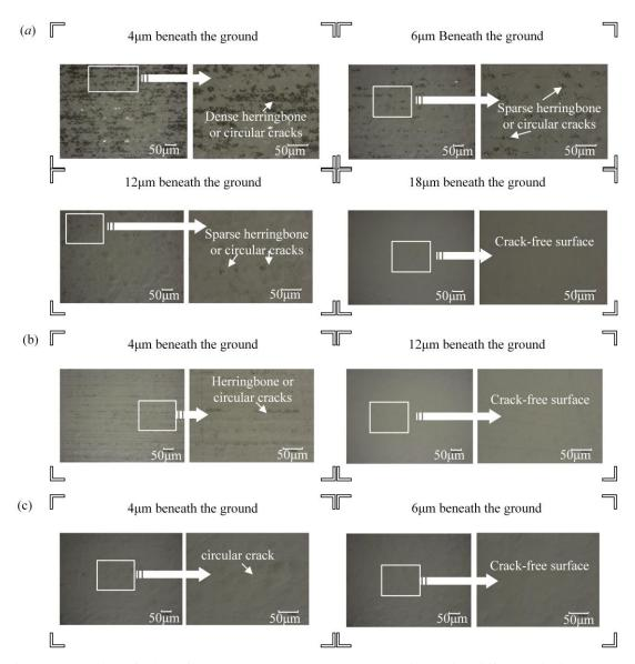
Fig. 7. Observation of sub-surface damages on samples ground obtained using different grinding depths (a)  $20\mu m$  (b)  $10\mu m$  and (c)  $2\mu m$
