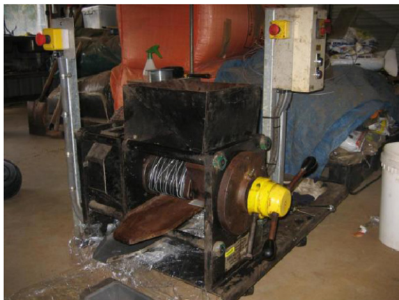
Fig. 2. Beauty leaf oil extraction using a screw press.
