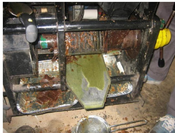
Fig. 2. Beauty leaf oil extraction using a screw press.
