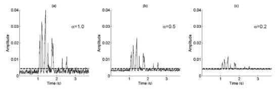
FIG 3. Example waveforms of compressed amplitude envelope with compression factor  $\alpha$  of values (a) 1.0, (b) 0.5, and (c) 0.2. The dashed line in each panel denotes the mean value of the amplitude envelope waveform.
