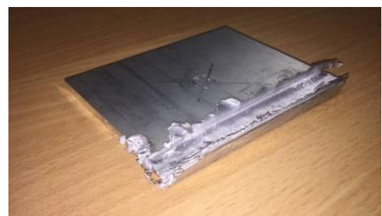
Fig. 6. Machining with an opposite spindle rotation direction
