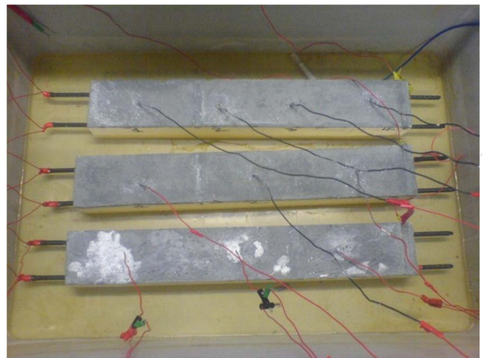
Fig. 3. Beams and circuit setup of cathodic polarization experiment
