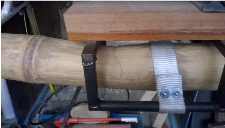
Figure 5 – Typical compression failure
