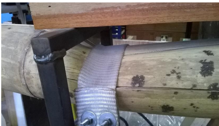
Figure 7 – Typical failure under loading straps
