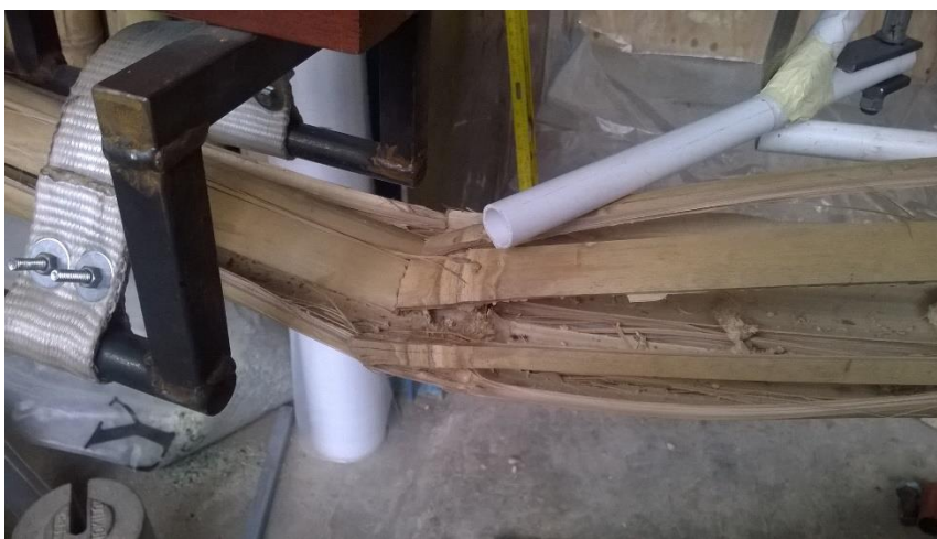
Figure 6 – Typical culm collapse
