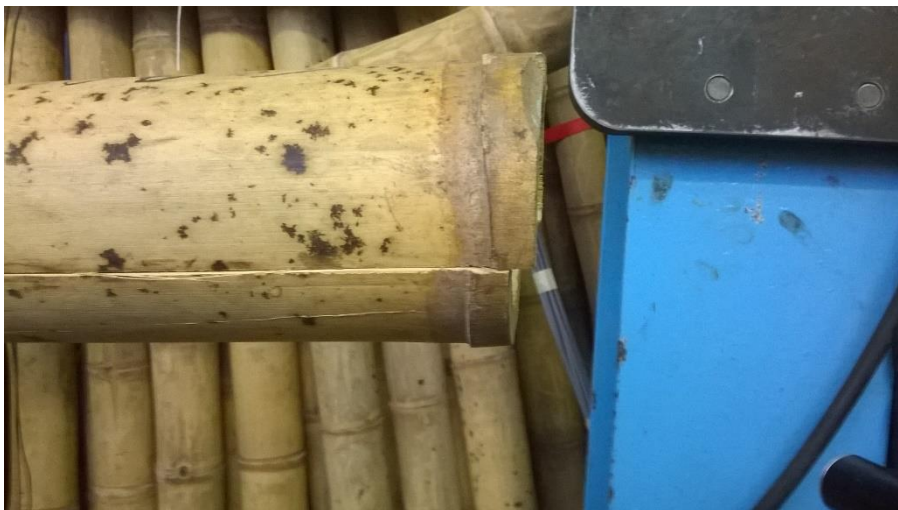
Figure 4 – Typical shear failure
