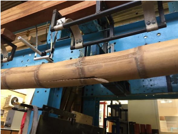
Figure 8 – Typical tension failure
