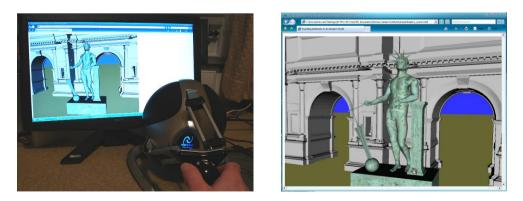
Figure 3. Ancient Rome on a haptic-enabled web browser with a Novint Falcon device
