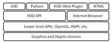
Figure 1. Architecture of a browser-based VE with haptics
