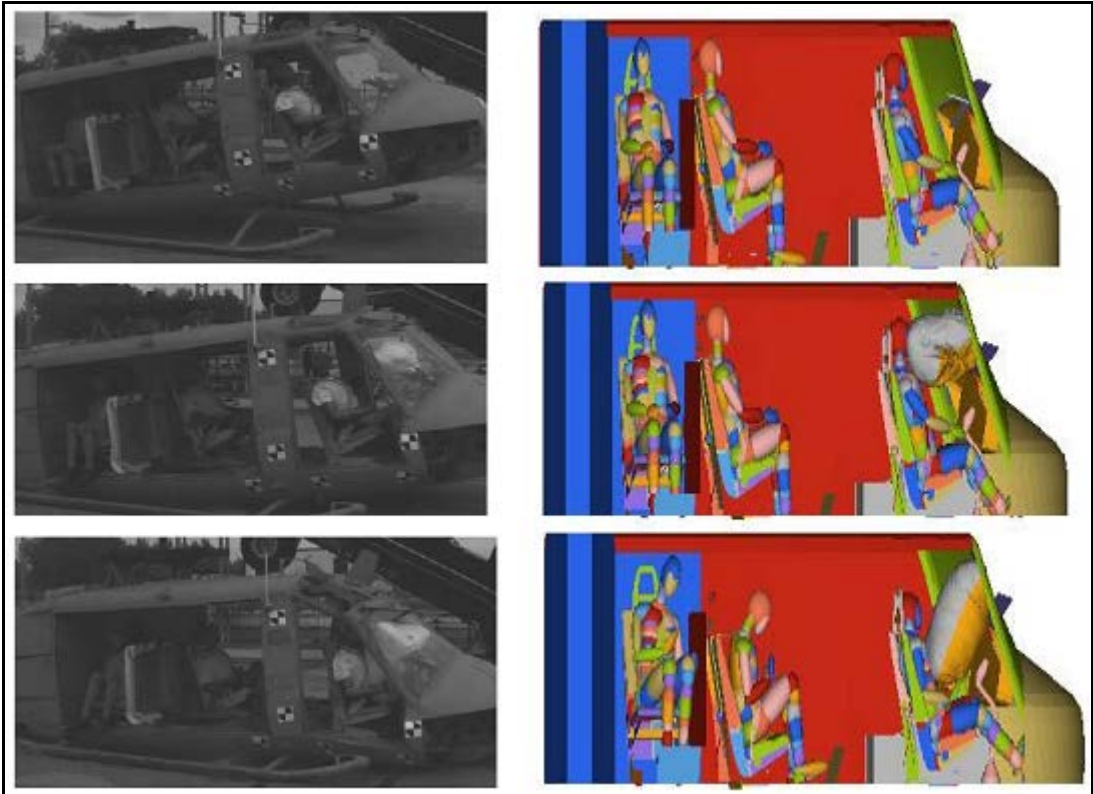
Figure 11 MADYMO Simulations of full-scale drop test with the Bell UH-1D cabin/cockpit model
