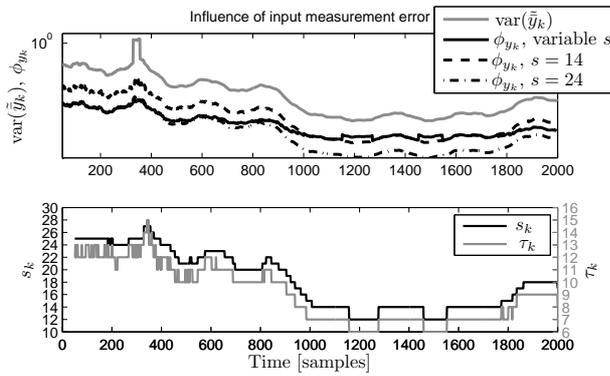
Figure 5: Parity space order and its influence on noise filtering
