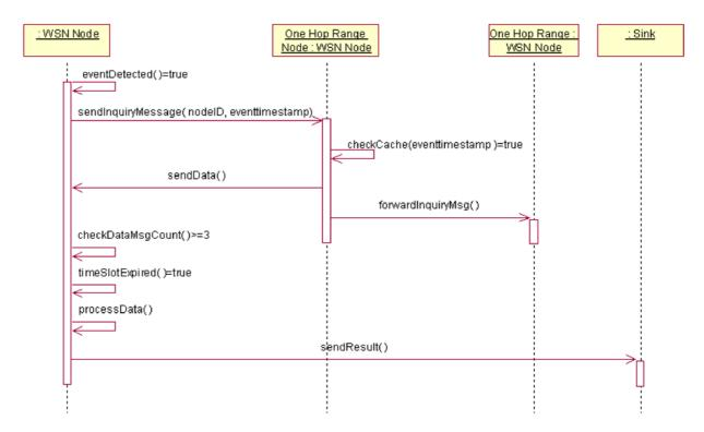
Fig. 11. Region-based approach to processing of acoustic data.
