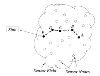
Fig. 1. A typical flat WSN architecture, taken from [18].
