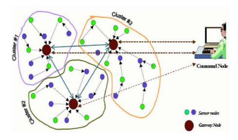
Fig. 2. A hierarchical, heterogeneous WSN architecture, taken from [24].
