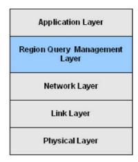
**Fig. 7.** DCQP Server-side architecture.
