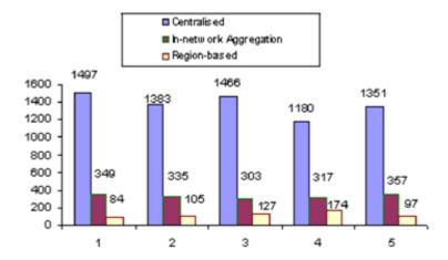
Fig. 13. Comparison of number of messages required for query resolution in a 100-node network.
