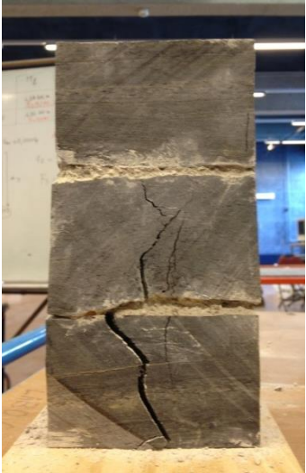
Figure 8: Sample of a schist triplet after failure.
