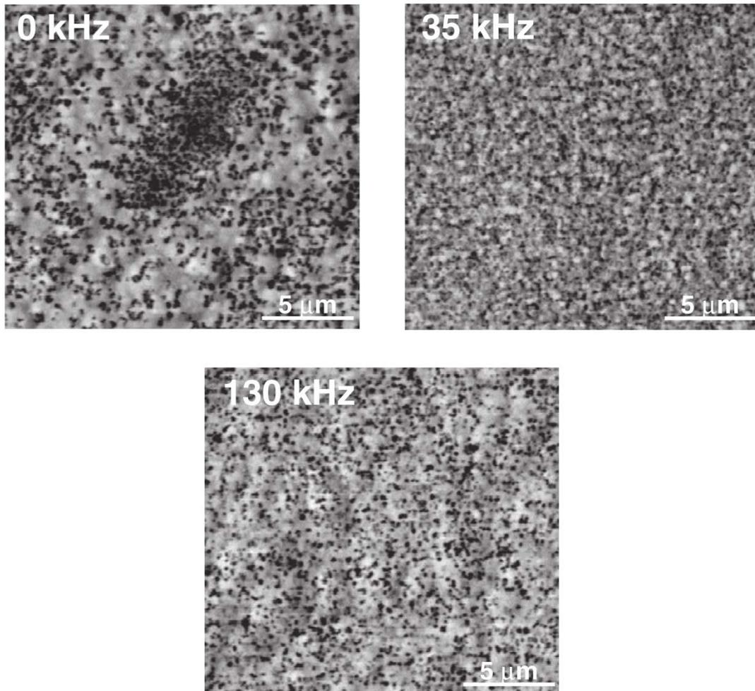
**Figure 7.** SEM (BSE) images of surface morphology of Ni-W/Al<sub>2</sub>O<sub>3</sub> composite coatings electrodeposited at a rotating speed of 340 rpm under different ultrasonic frequencies. Adapted from Ref. [58], with permission from Elsevier.
