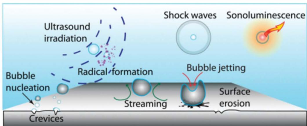
**Figure 2.** Schematic representation of the main effects of cavitation induced by ultrasound irradiation. Adapted from Ref. [9], with permission of The Royal Society of Chemistry.
