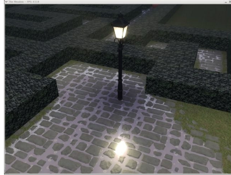
Figure 8: Achieving a mirror effect by rendering the geometry twice [AM07].
