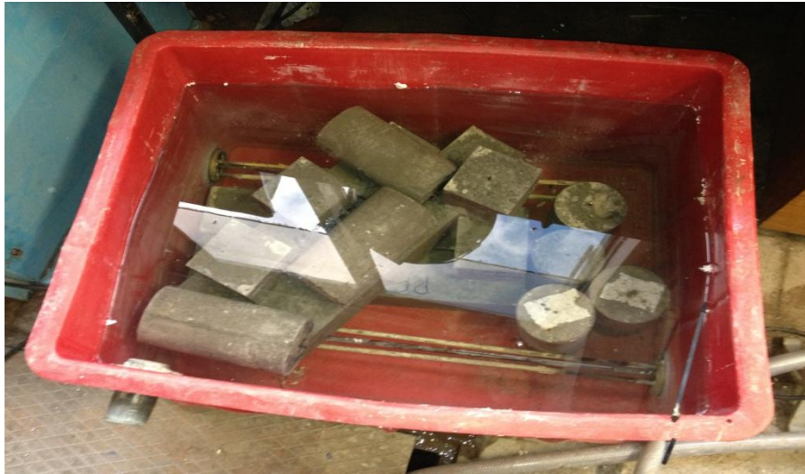
Figure 1. Hot curing of concrete specimens
