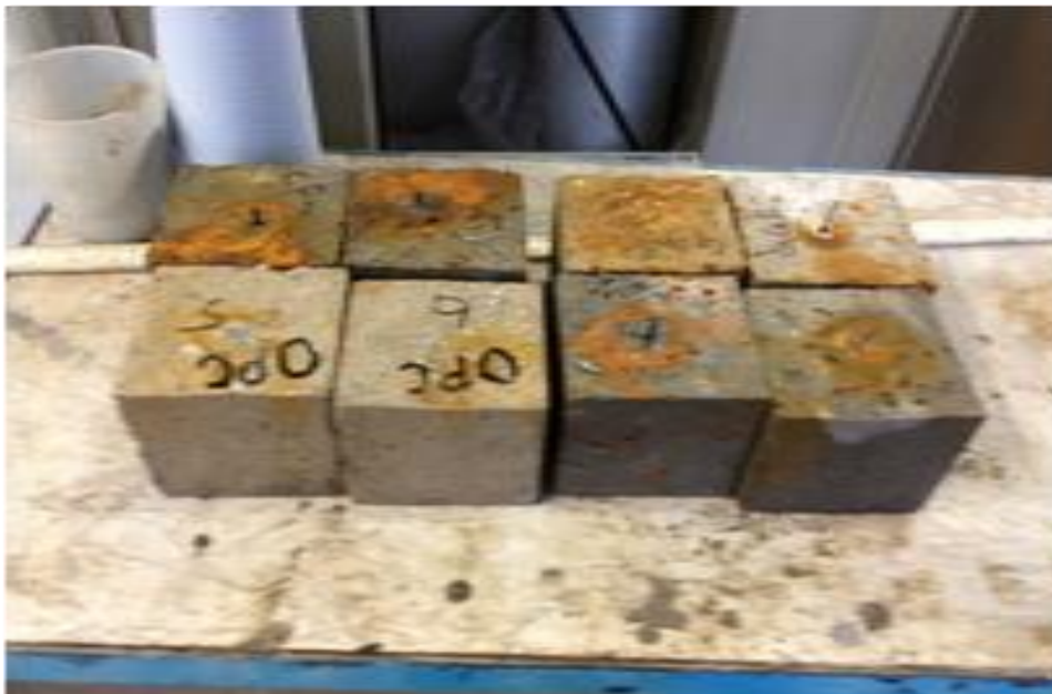
Figure 5. Concrete specimens after accelerated corrosion test
