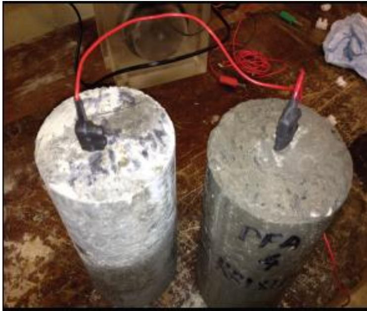
Figure 4. Concrete specimens before accelerated corrosion test
