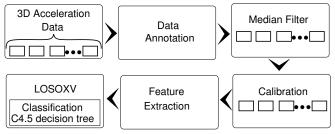
Fig. 2. Data processing flow for system training.
