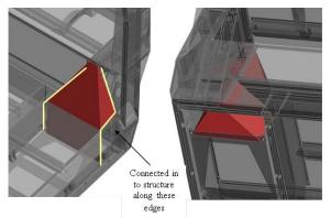
Figure 14 Concept 1 - Gusset reinforcement
