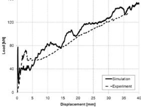
Figure 5 Comparison of experimental load displacement curve with simulation results [3]
