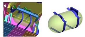
Figure 13 New hydrogen tank mounting strategy
