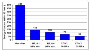
Figure 3 Energy content in 60 litre tank [1]
