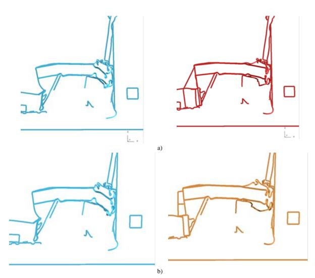
Figure 16 Comparision between the deformed shape of the rear of the Microcab a) Baseline - Concept 1, b) Baseline - Concept 2
