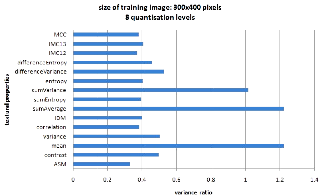
Figure 4.5 Variance ratio bar graph for training images with 300x400 pixels image size and 8 quantisation levels
