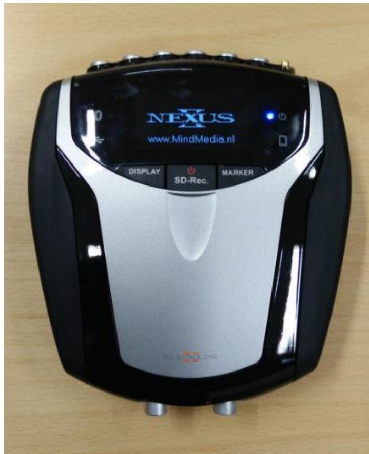
Figure 7. NeXus-10 MkII multichannel biofeedback device
