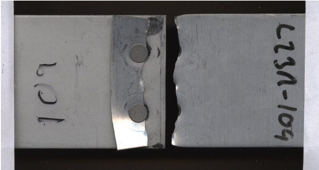
Figure 20: Eyebrow failure with 5.5 KN maximum load at 0.18 million cycles
