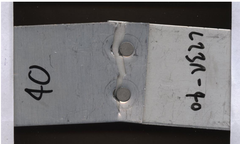
Figure 16: Eyebrow failure at maximum load of 3 KN at 1.63 million cycles
