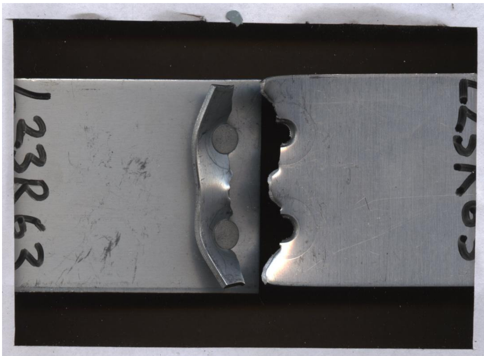
Figure 22: 3-9 failure mode at maximum load 8kN and 54000 cycles
