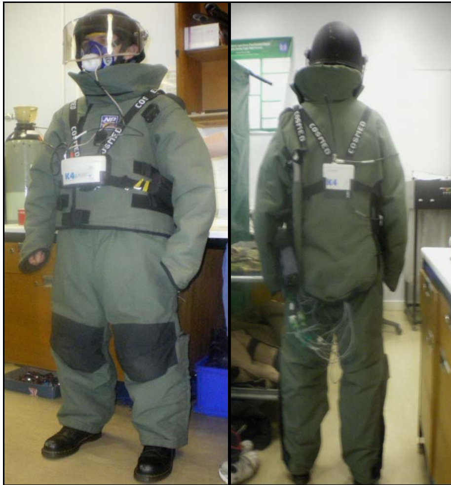
Figure 3. 6: The 3010 Ergotec EOD ensemble with instrumentation prior to entering the experimental chamber.
