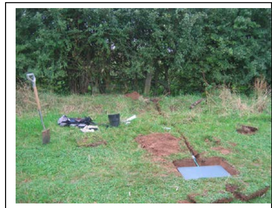
Figure 2.5 Installation of pressure pads
