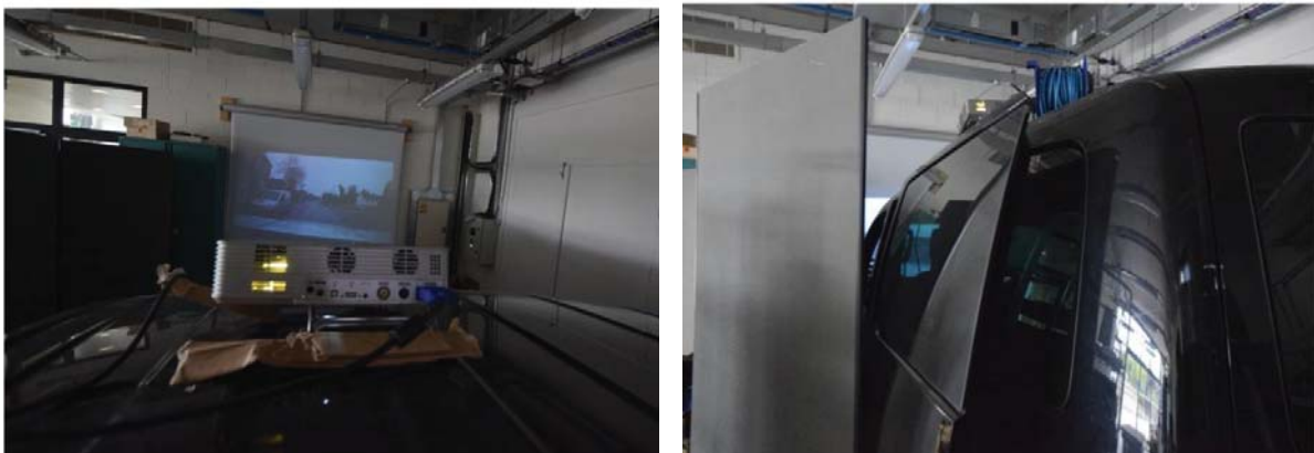
Fig. 1. Simulator used in this study. The projector was placed above the Nissan vehicle to allow the projection to be displayed onto the wall (left) and large grey panels blocking the vehicle's windows were used to prevent environmental distraction (right).
