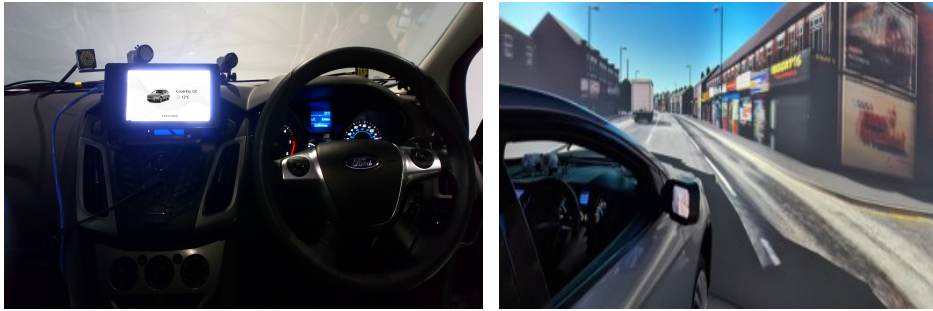
Figure 1: (left) Driver's view of the dashboard and HMI used for activating the automation (right) Driver in-the-loop simulator and its 4.75 meter, 270 degree curved screen.
