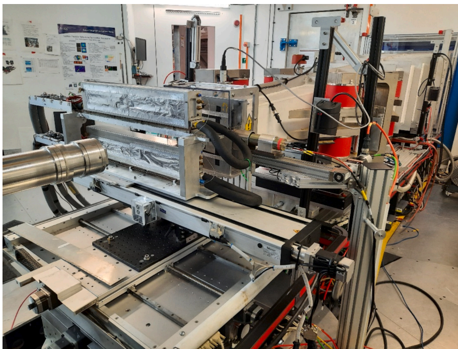
Fig. 1. Experiment setup used for the SANS experiment at LARMOR instrument. The sample is placed in the neutron beam of aperture 6*6 mm, coming from Target station 2 at ISIS facility. The transmitted beam is stopped by a beam stop. The scattered beam is detected by using the He 3 detector placed behind the sample. SANS measurement was done for 15 \mu A and TRANS measurement was done for 5 \mu A.
