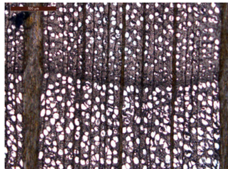
Fig. 2.9. Transverse section through beech. Morwenna Spear © Chris Miles.
