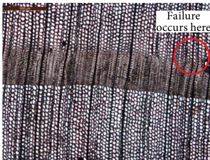
Fig. 2.8. Transverse section through a Scots pine. Morwenna Spear © Chris Miles.
