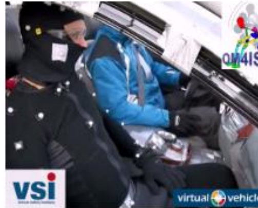
Left: 50 th Percentile volunteer (OM4IS) Right: Standard Simcenter Madymo AHM positioned on rigid seat
