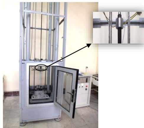
Figure 9. Drop-weight test device and the accelerometer
