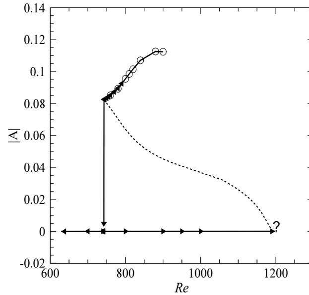
FIGURE 7. Hysteretic behavior described by the fluctuation of the integral of velocity magnitude throughout the domain as a function of  $Re$  at  $\beta = 1$ , reducing  $Re$  from an unsteady flow ( $\blacktriangleleft$ ) and increasing  $Re$  from a steady flow ( $\blacktriangleright$ ) give different  $Re_c$ .  $|A| = 0$  indicates steady flow solution.
