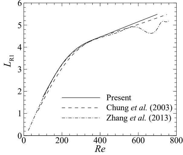
FIGURE 4. Length of the first recirculation bubble ( $L_{R1}$ ) against Reynolds number ( $Re$ ) for  $\beta = 1$ , comparing the present results to those of Zhang & Poth erat (2013) and Chung *et al.* (2003).
