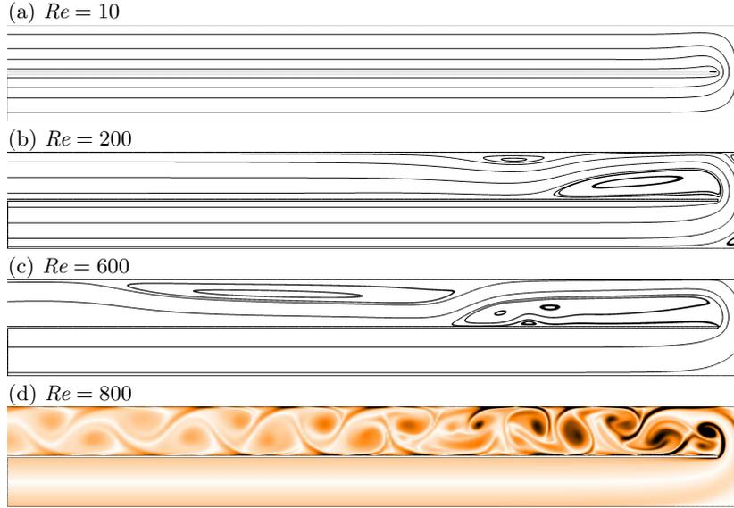
FIGURE 5. Streamlines of steady two-dimensional base flow at (a)  $Re = 10$ , (b)  $Re = 200$ , (c)  $Re = 600$  and (d) flooded contours of vorticity magnitude at  $Re = 800$  for  $\beta = 0.5$ . In (d), white represents zero vorticity (no rotation), and darker shading denotes arbitrarily higher vorticity magnitude levels.
