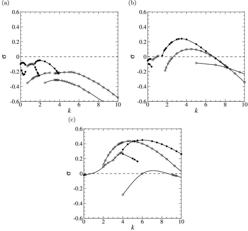
FIGURE 13. Growth rates of leading eigenmodes plotted against spanwise wavenumber at  $\beta = 0.5$  for (a)  $Re = 200$ , (b)  $Re = 400$  and (c)  $Re = 600$ . Solid symbols represent real leading eigenvalues, meanwhile hollow symbols represent complex-conjugate pairs of leading non-real eigenvalues.
