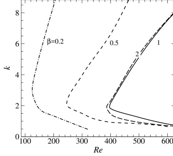
FIGURE 16. Marginal stability curves for sharp 180-degree bend flow with  $\beta = 0.2, 0.5, 1,$  and  $2$ . Regions on the right of the curves represent flow conditions that are linearly unstable to three-dimensional perturbations for that particular  $\beta$ .
