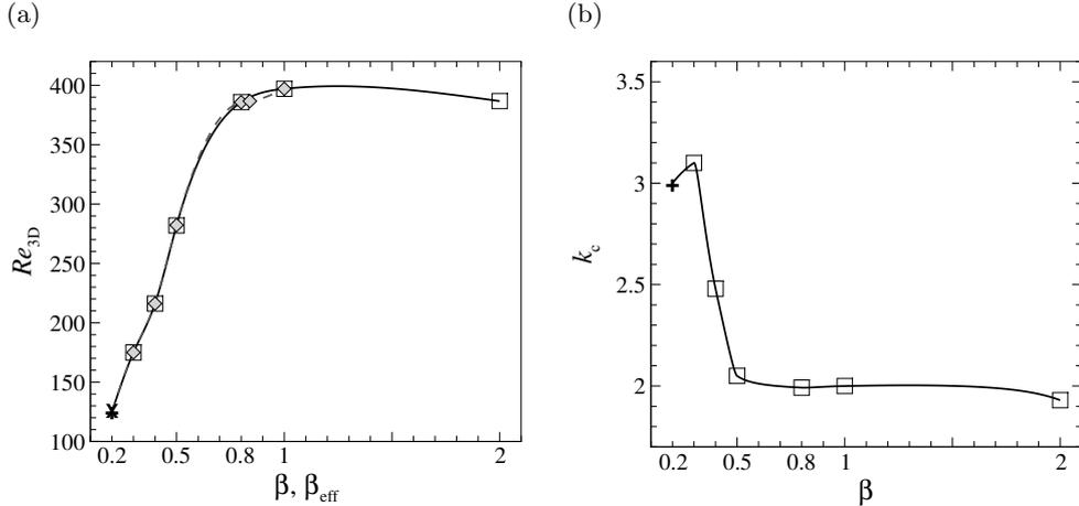
FIGURE 15. Critical (a) Reynolds number and (b) wavenumber as a function of opening ratio. In (a) the critical Reynolds number is also plotted against effective opening ratio  $\beta_{eff}$ . For  $\beta$  data, synchronous modes and oscillatory modes are represented respectively by “□” and “+”. For  $\beta_{eff}$  data, synchronous and oscillatory modes are respectively represented by “◇” and “×”.
