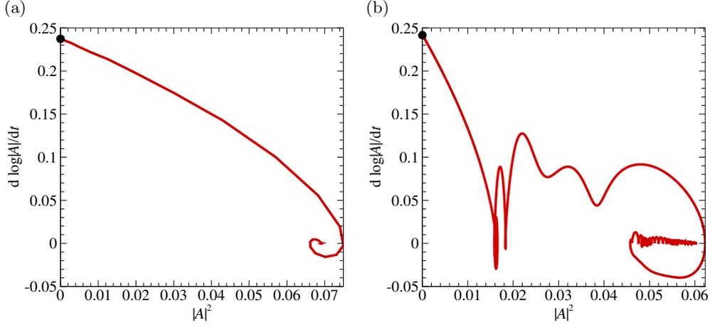
FIGURE 24. The time derivative of mode amplitude logarithm plotted against the square of the amplitude for (a)  $\beta = 0.2$ ,  $Re = 160$ ,  $k = 4$  and (b)  $\beta = 0.5$ ,  $Re = 400$ ,  $k = 3.5$  demonstrating supercritical behaviour. The solid circle symbol represents the linear stability analysis predicted growth rate.
