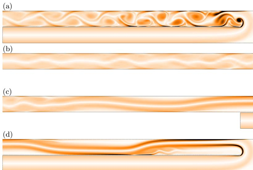
FIGURE 8. Flooded contours of vorticity magnitude demonstrating unsteady saturated flows for (a)  $Re = 800$  at  $\beta = 1$  (which was initiated from rest), and (b)-(d)  $Re = 1152$  at  $\beta = 1$  (which was initiated from a saturated steady-state flow solution at a lower Reynolds number). Contour levels are as per figure 5(d). (b), (c) and (d) show domain segments  $-45 \leq x \leq -29$ ,  $-30 \leq x \leq -14$  and  $-15 \leq x \leq 1$ , respectively.
