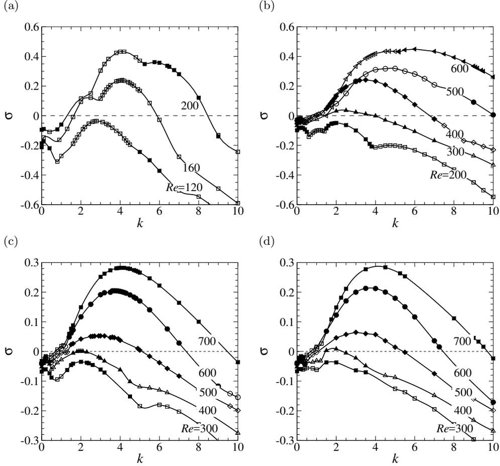
FIGURE 12. Growth rates of leading eigenmodes as a function of spanwise wavenumber  $k$  for (a)  $\beta = 0.2$  and  $Re \leq 200$ , (b)  $\beta = 0.5$  and  $Re \leq 600$ , (c)  $\beta = 1$  and  $Re \leq 700$ , and (d)  $\beta = 2$  and  $Re \leq 700$ . Solid symbols represent real leading eigenvalues, while hollow symbols represent complex-conjugate pairs of non-real leading eigenvalues. Solid lines connect all dominant leading eigenvalues from several branches of the same Reynolds number.
