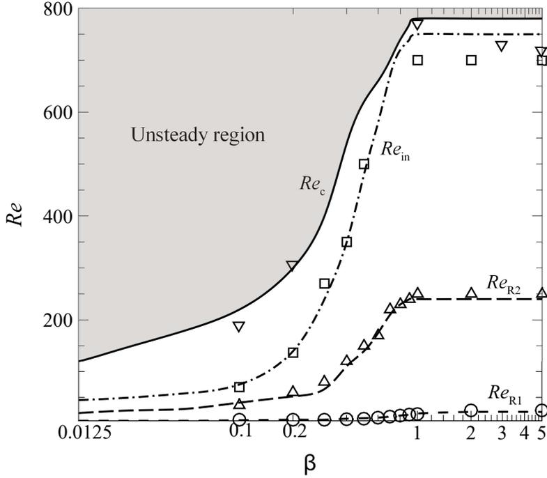
FIGURE 6. Reynolds number where primary recirculation bubble  $Re_{R_1}$ , secondary recirculation bubble  $Re_{R_2}$  and inside recirculation bubble  $Re_{in}$  start to appear in the two-dimensional flow.  $Re_c$  is the transition from steady to unsteady. The lines are from current study and the symbols are results from Zhang & Poth erat (2013).  $\circ$ ,  $\triangle$ ,  $\square$  and  $\nabla$  represent  $Re_{R_1}$ ,  $Re_{R_2}$ ,  $Re_{in}$  and  $Re_c$ , respectively.
