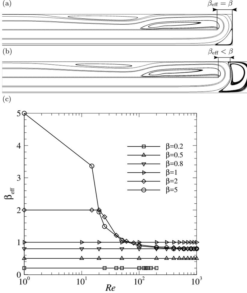
FIGURE 11. Streamlines of steady two-dimensional flow for  $Re = 600$ , (a)  $\beta = 1$  and (b)  $\beta = 2$ . A big recirculation bubble appears at the far end of the wall when  $\beta > 1$  causing the effective bend opening ratio to be lesser than the actual opening.  $\beta_{\text{eff}}(Re)$  is plotted in (c) for several value of  $\beta$ .
