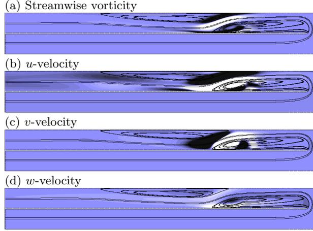
FIGURE 20. Structure of the real part of the leading eigenmode at  $\beta = 0.5$ ,  $Re = 400$  and  $k = 0.2$  depicted on the plane  $z = 0$ : flooded contours of (a) streamwise vorticity and (b)  $u$ , (c)  $v$  and (d)  $w$ -velocity overlaid with the base flow streamlines. For clarity, only the vicinity of the bend is shown. Dark-mid-light shading denotes negative-zero-positive levels, respectively.
