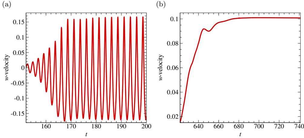
FIGURE 22. Time histories of  $w$ -velocity measured at a local point  $(x, y, z) = (-2, 0.52, 1)$ . Because  $w$  is zero in the underlying two-dimensional base flow, non-zero  $w$  is an indicator for three-dimensional flow development. In (a)  $\beta = 0.2$ ,  $Re = 160$  and the three-dimensional spanwise domain wavenumber is  $k = 4$ . In (b)  $\beta = 1$ ,  $Re = 600$  and  $k = 4.5$ .
