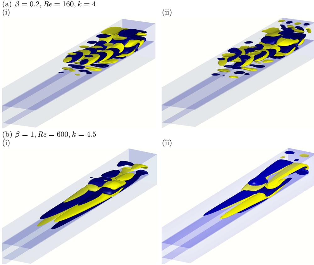
FIGURE 23. Visualisation of the three-dimensional disturbances via iso-surface plots of the (streamwise)  $x$ -component of vorticity for (a)  $\beta = 0.2, Re = 160, k = 4$  and (b)  $\beta = 1, Re = 600, k = 4.5$ . (i) shows the leading eigenmode predicted by the linear stability analysis, and (ii) shows the saturated state of a three-dimensional DNS simulation. The saturated solution in (a ii) is oscillatory, and in (b ii) is steady-state.
