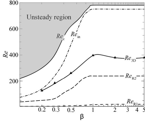
FIGURE 18. Parameter space for flow regimes and leading peak eigenvalues of three-dimensional stability. The onset of three-dimensional instability is represented by  $\triangle$  symbols. Lines are included for guidance, and the shaded region shows the parameter values exhibiting unsteady two-dimensional solutions.
