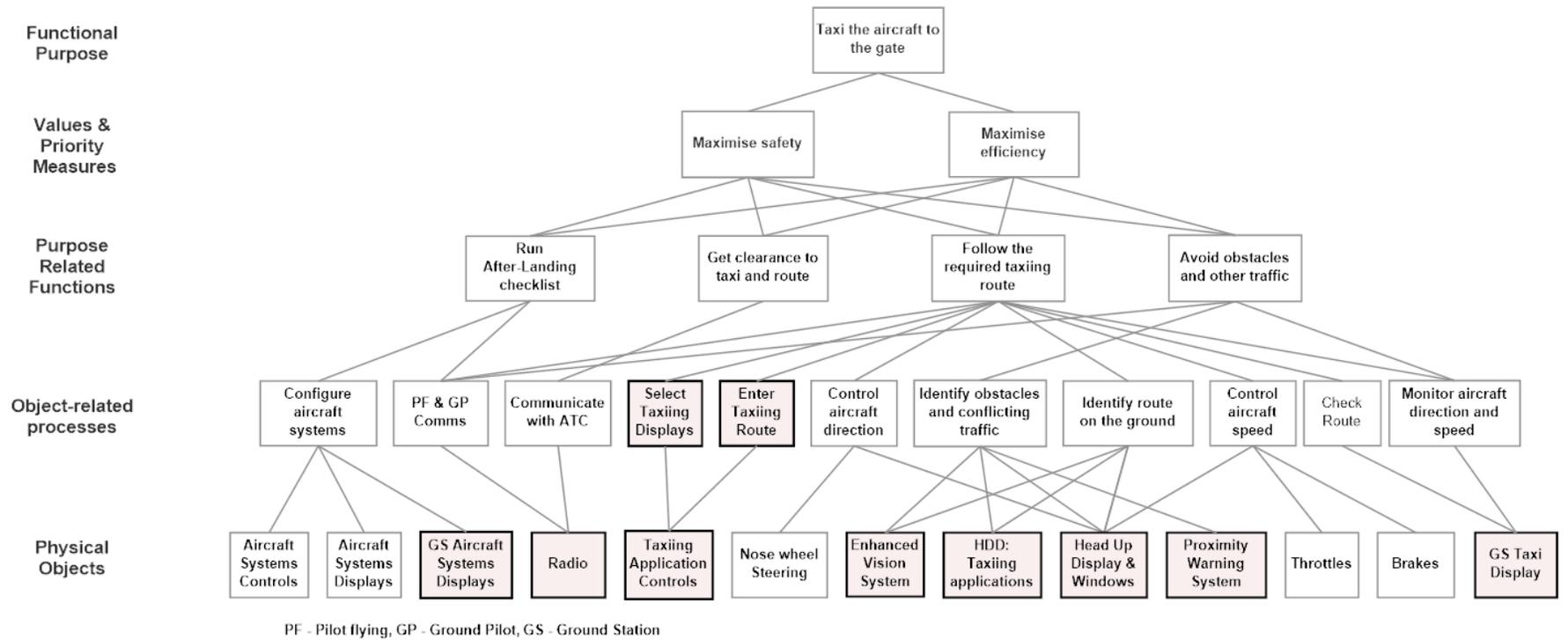
**Fig 3** WDA abstraction hierarchy for taxiing the aircraft to the gate for single pilot operations incorporating new technologies and GP-based functions.
