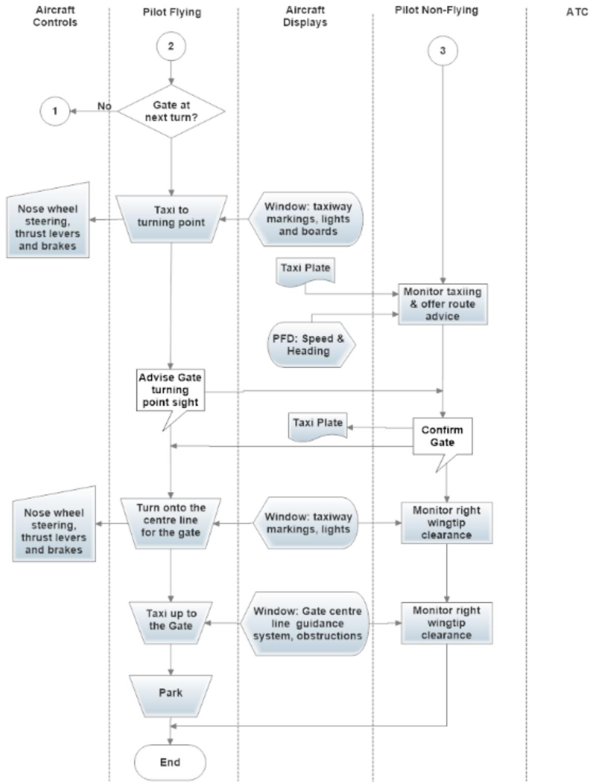
Fig 1b OECD for taxiing the aircraft to the gate for two pilot operations (continued).
