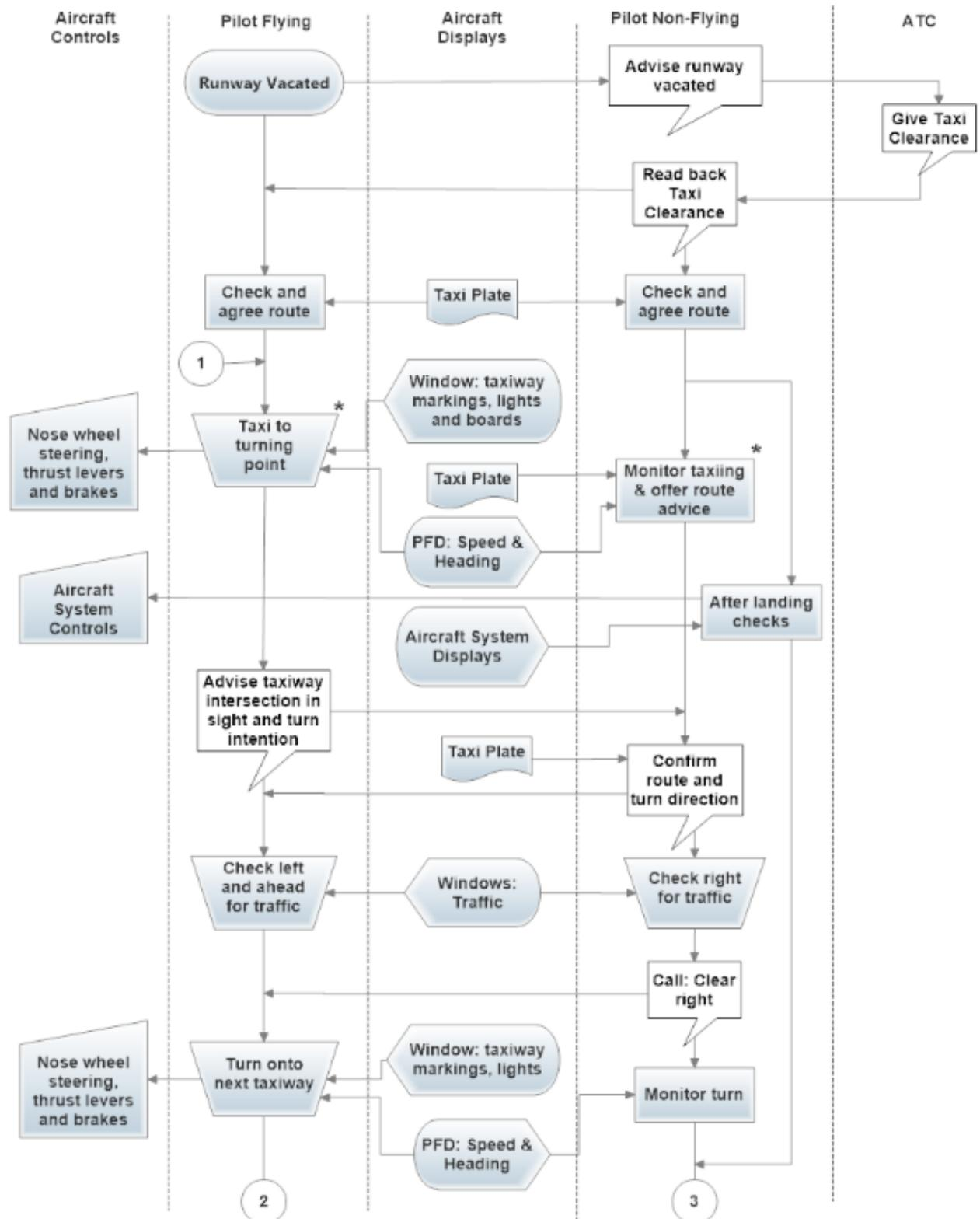
Fig 1a OESD for taxiing the aircraft to the gate for two pilot operations (baseline)
