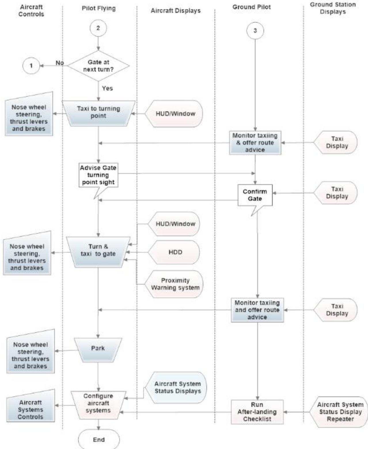
Fig 4b OECD for taxiing the aircraft to the gate for single pilot operations incorporating new technologies and GP-based functions (continued).
