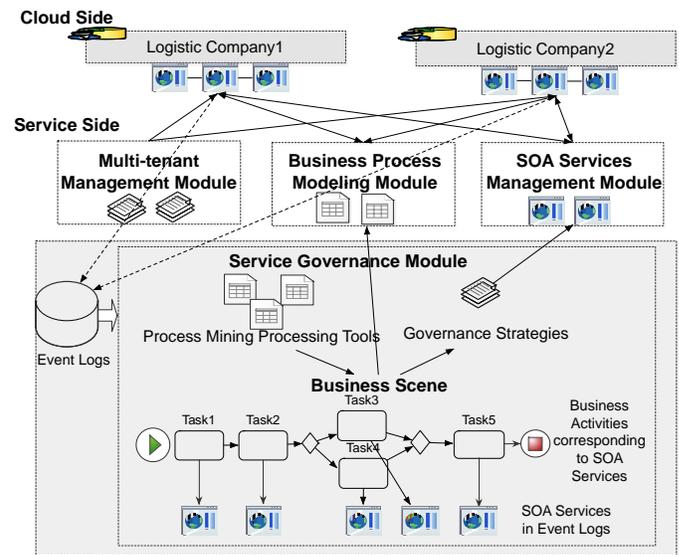
Figure 8. Architecture of the cloud logistic management platform
