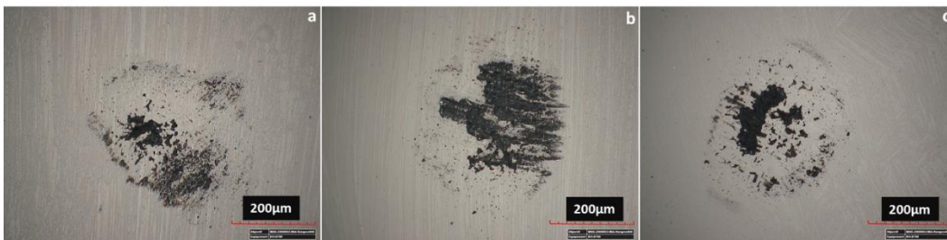
Fig. 5 - Optical microscope surface of testing alumina balls after the dry sliding friction test. (a) electroless NiB without ultrasound, (b) electroless NiB with 20 kHz frequency and 0.058 W/cm 3 energy density ultrasound, (c) electroless NiB with 35 kHz frequency and 0.065 W/cm 3 energy density ultrasound.
