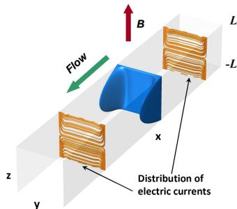
Fig. 1: Flow geometry of Hunt's flow in a square duct. Laminar velocity distribution with perfectly conducting Hartmann- and perfectly insulating parallel-walls is shown at  $Ha = 100$  (blue); also shown are the streamlines of electric current density (brown).
