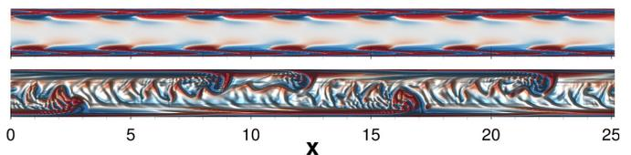
Fig. 5: Instantaneous snapshots of flow fields at  $Re = 1000$  shown for incremental (top) and decremental (bottom) simulations. The flow patterns are visualized by the vertical vorticity component  $\omega_z$  in the  $(x, y)$ -mid-plane ("blue-red" gradient corresponds to "negative-positive" ranges of  $\omega_z$ ).
