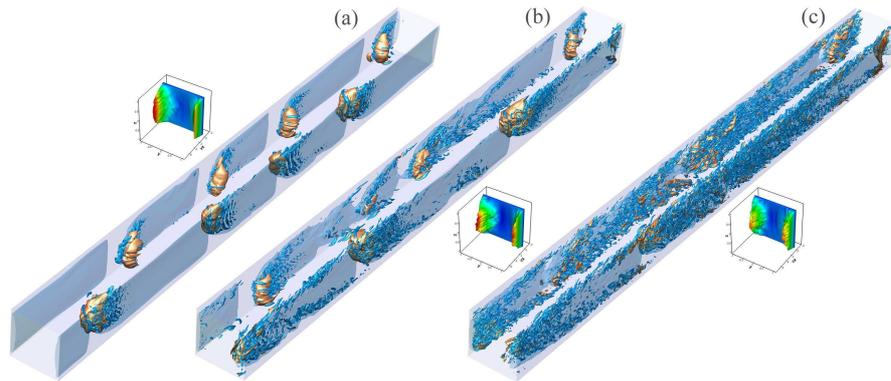
Fig. 6: Evolution of jet detachments versus  $Re$ , instantaneous snapshots of flow fields are visualized at  $Re = 2000$  (a),  $3000$  (b) and  $4000$  (c). Shown are the isosurfaces of full-scale streamwise velocity  $U_x$  at the side walls (light blue), TKE of transverse velocity  $u_y^2 + u_z^2$  (gold) and  $\lambda_2$  criterion (cyan). The inserts show velocity profiles in the  $(y, z)$ -section at  $x = L_x/2$ .
