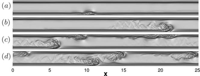
Fig. 3: Temporal evolution of jet detachments at  $Re = 1630$  and  $Ha = 100$ . Full streamwise velocity  $U_x$  is shown in the  $(x, y)$ -mid-plane at  $z = 0$ , corresponding to four phases of evolution (every 7 convective units), beginning from a single event on one side-wall to the fully developed unsteady behavior (from top to bottom). Flow direction is from left to right, magnetic field vector is perpendicular to the  $(x, y)$ -plane.
