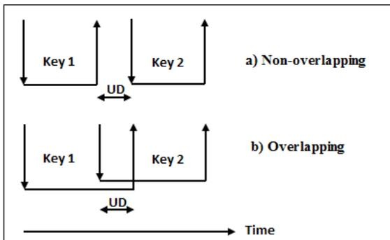
Fig. 1. Negative UD caused by overlapping keystroke events.
