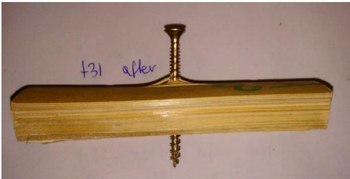
Figure 10: typical withdrawal failure mode
