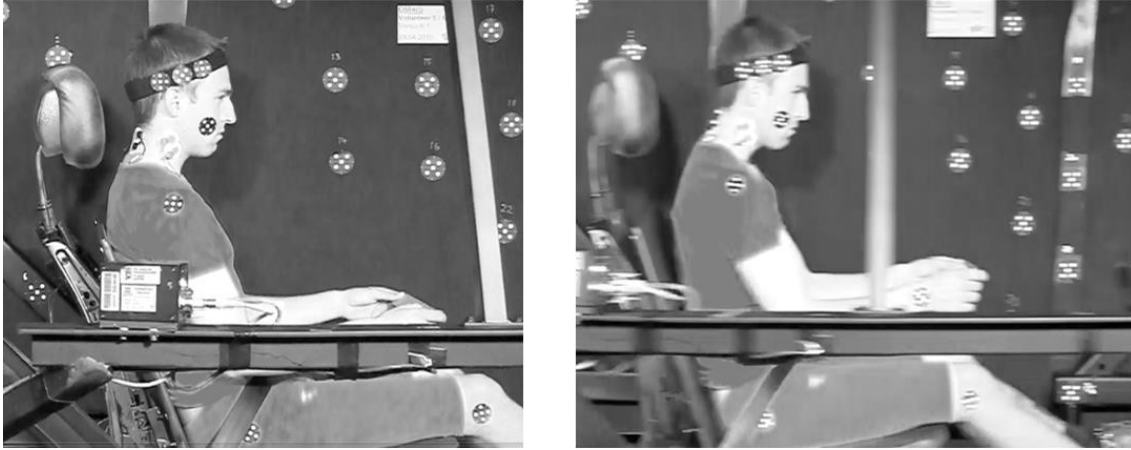
Figure 5: A typical OM4IS frontal sled test [20]
