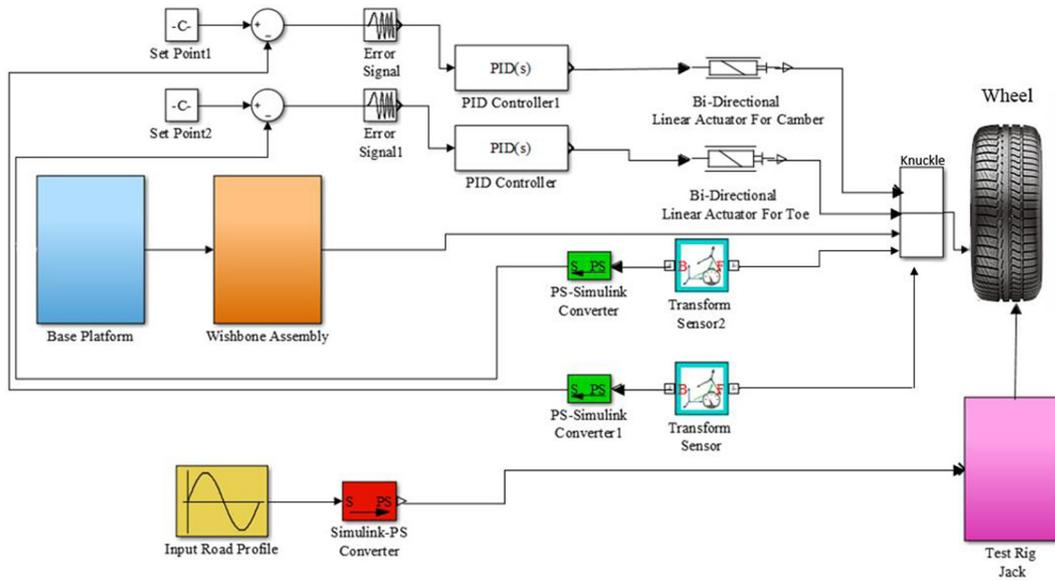
Fig. 6. Simulink block diagram of adaptive suspension system.
