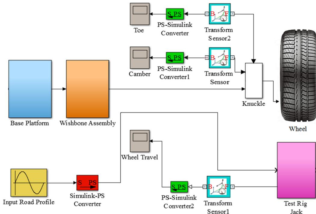
Fig. 5. Simulink block diagram of passive suspension system.
