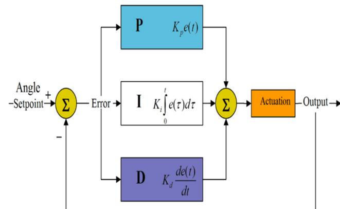
Fig. 7. Schematic of the PID control system.
