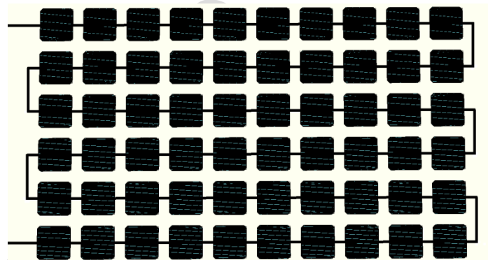
Figure 2(a). Traditional PV module configuration for PVSS
