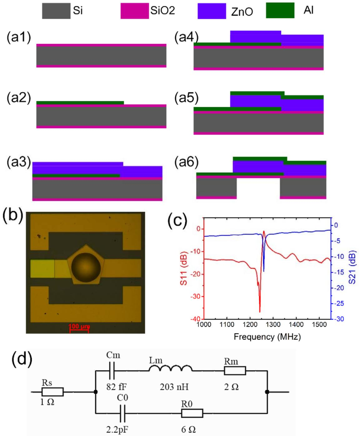
Figure 1. The FBAR microfabrication process (a): (a1) a silicon wafer with a ~1 μm SiO<sub>2</sub> film, (a2) shaped bottom electrode, (a3) deposited ZnO, (a4) exposed the bottom electrode, (a5) graphic top electrode, (a6) etch the back side silicon. Microphoto image of the fabricated FBAR device (b), the obtained S-parameters of the device (c), and the MBVD model circuit and specific values of variables extracted from the S-parameters (d).
