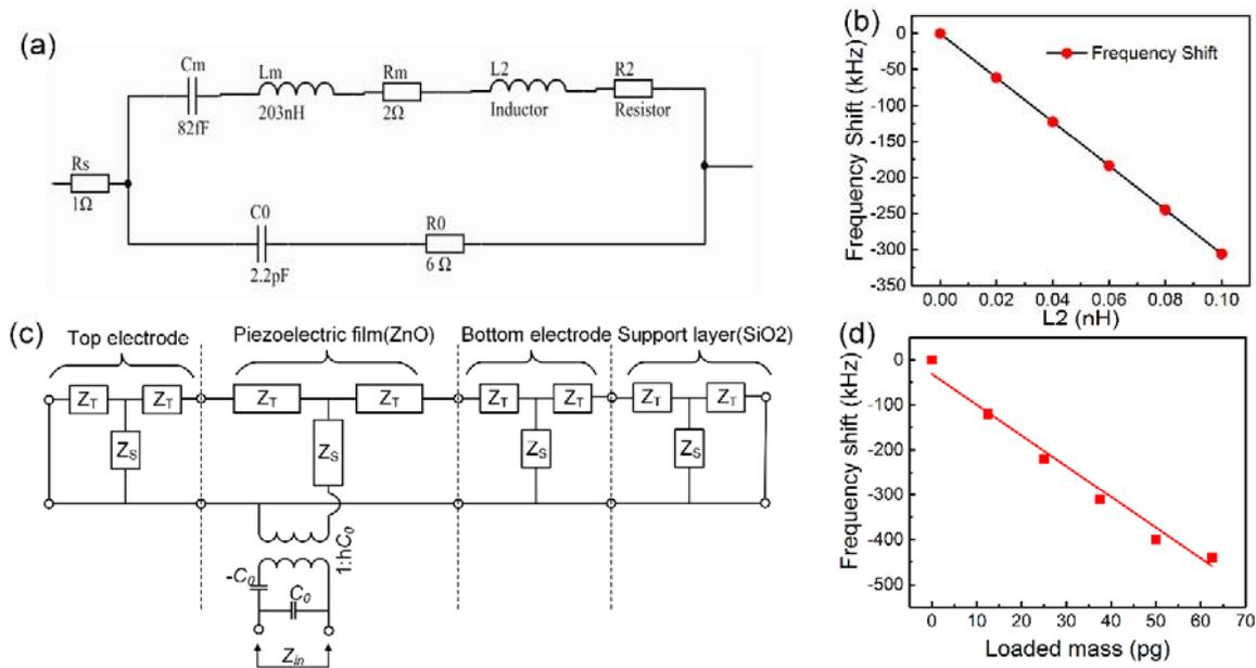
Figure 5. (a) the simulated relationship between the introduced inductor by the mass loading and the output frequency of the oscillator; (b) the MBVD model of FBAR device with mass loading, (c) the Mason's equivalent circuit of FBAR device, and (d) the theoretical frequency response of the FBAR based on Mason's model.
