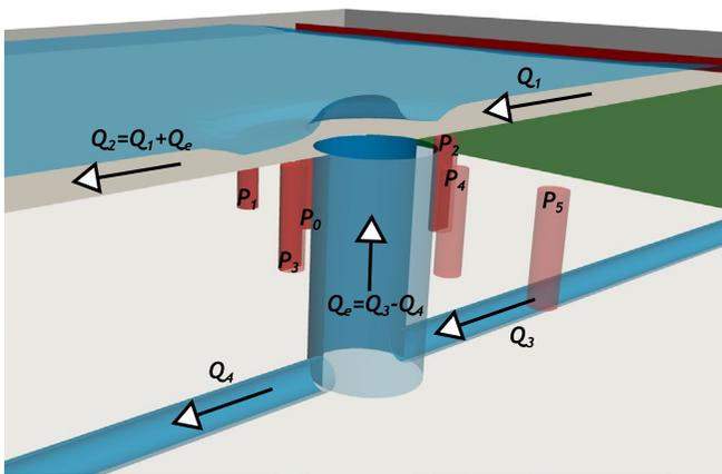
Figure 2. 3D representation of manhole/surface exchange location with surface inflow ( $Q_1$ ), surface outflow ( $Q_2$ ), sewer inflow ( $Q_3$ ) and sewer outflow ( $Q_4$ ) and depth measurement locations ( $P_x$ ) around the manhole.
