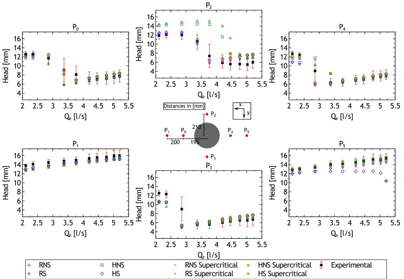
**Figure 4.** Comparison between the experimental observations and numerical hydraulic heads at each measurement location. The (temporally averaged) experimental data points are bounded by the 1st and 3rd quartile of the measured time series data.
