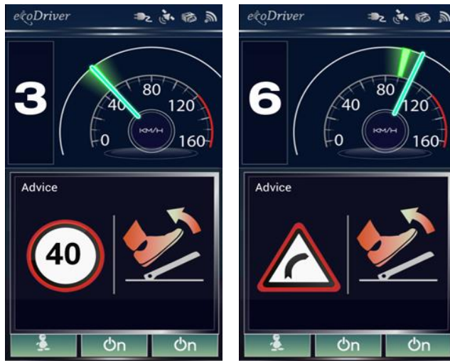
Fig.1. FeDS advice for speed limit event (left) and FeDS advice for curve event (right).
