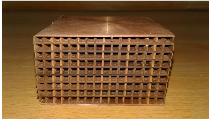
Fig. 6 Fabricated squarebore microhole3 (Cu) structure
