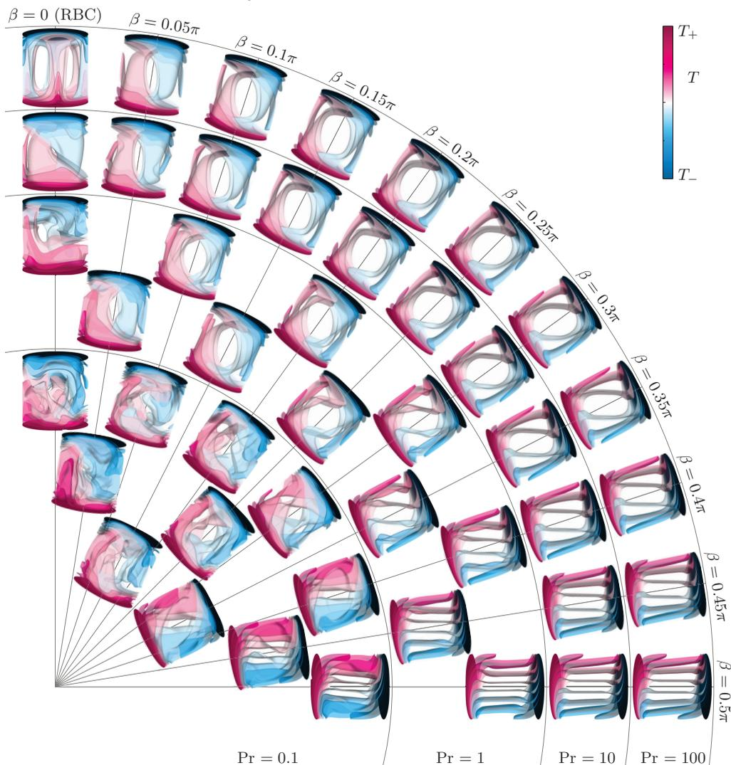
FIGURE 2. Isosurfaces of the instantaneous temperature fields in inclined convection in cylindrical containers, filled with a fluid of  $Pr = 0.1$ ,  $Pr = 1$ ,  $Pr = 10$  or  $Pr = 100$ , for  $Ra = 10^6$  and different inclination angles from  $\beta = 0$  to  $\beta = 0.5\pi$ , as obtained in our DNS. Shown are ten isosurfaces that are equidistantly distributed between the heated ( $T_+$ ) and cooled ( $T_-$ ) cell boundaries.
