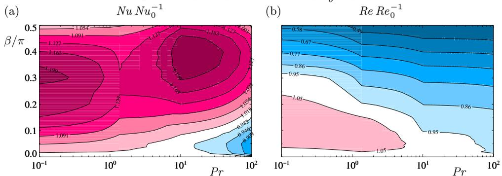
FIGURE 7. Phase diagrams for (a)  $Nu Nu_0^{-1}$  and (b)  $Re Re_0^{-1}$  in the  $(Pr, \beta)$  plane, showing the regions of a relative increase (pink) or decrease (blue) of the Nusselt and Reynolds numbers with respect to the RBC case ( $\beta = 0$ ), as it was obtained in the DNS.
