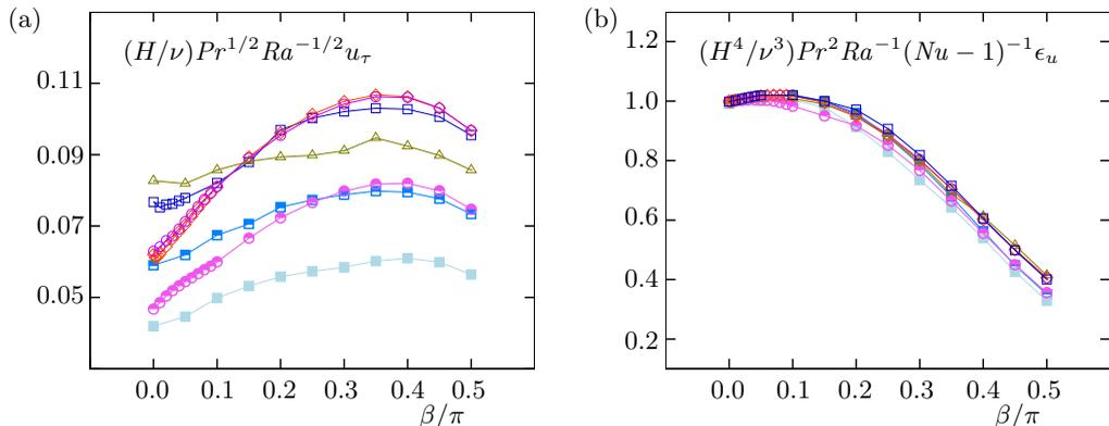
FIGURE 6. Normalized (a) friction velocity  $u_\tau$ , averaged in time and over the top and bottom plates, and (b) time- and volume-averaged kinetic dissipation rate  $\epsilon_u$ , in inclined convection in a cylinder of the aspect ratio 1, for  $Pr = 0.1$  (triangles),  $Pr = 1$  (squares),  $Pr = 10$  (circles) and  $Pr = 100$  (diamonds), and  $Ra = 10^6$  (open symbols),  $Ra = 10^7$  (half filled symbols) and  $Ra = 10^8$  (filled symbols), as functions of the inclination angle  $\beta$ .
