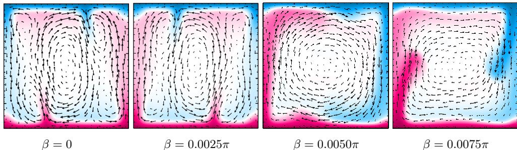
FIGURE 3. Changing of the instantaneous temperature fields with a small inclination angle  $\beta$  for  $Pr = 100$  and  $Ra = 10^6$ . Colour scale as in figure 2.
