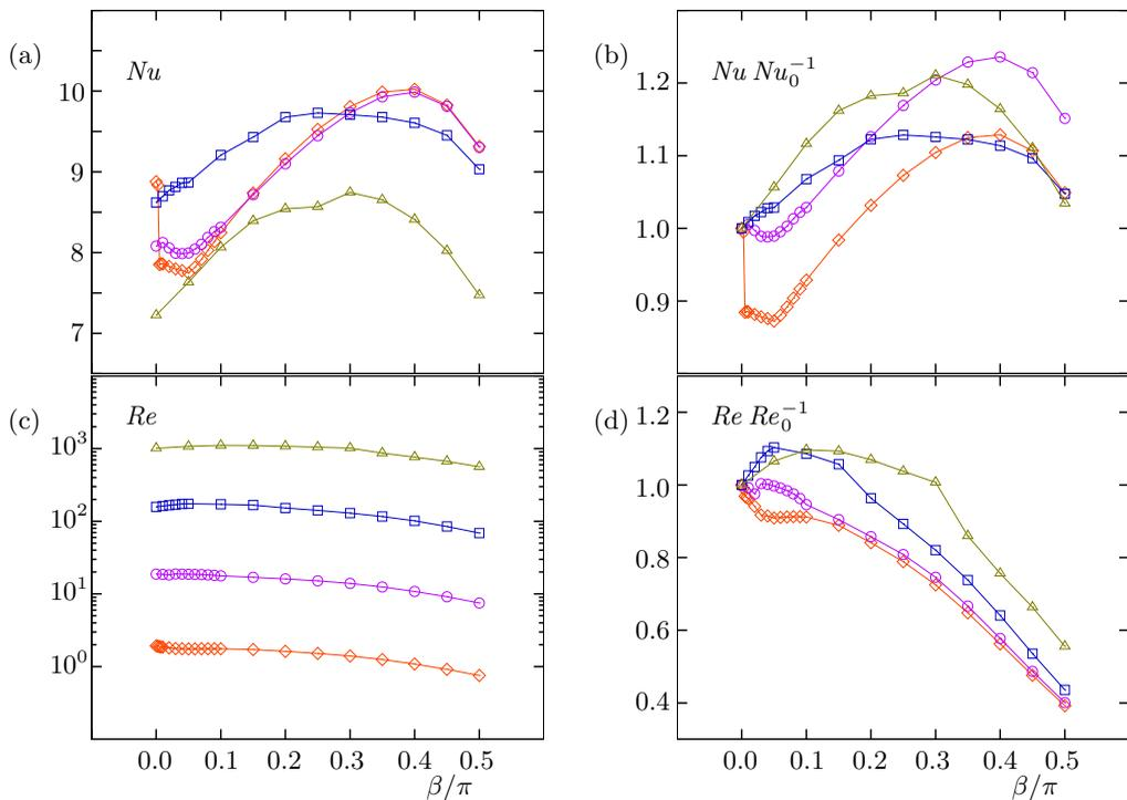
FIGURE 4. Absolute (a, c) and normalized (b, d) with the corresponding values for RBC ( $\beta = 0$ ) Nusselt numbers (a, b) and Reynolds numbers (c, d) in inclined convection in a cylinder of the aspect ratio 1, for  $Ra = 10^6$  and  $Pr = 0.1$  (triangles),  $Pr = 1$  (squares),  $Pr = 10$  (circles) and  $Pr = 100$  (diamonds), as functions of the inclination angle  $\beta$ .
