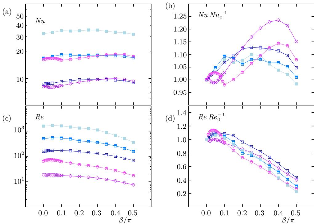
FIGURE 5. Absolute (a, c) and normalized (b, d) with the corresponding values for RBC ( $\beta = 0$ ) Nusselt numbers (a, b) and Reynolds numbers (c, d) in inclined convection in a cylinder of the aspect ratio 1, for  $Pr = 1$  (squares) and  $Pr = 10$  (circles), and  $Ra = 10^6$  (open symbols),  $Ra = 10^7$  (half filled symbols) and  $Ra = 10^8$  (filled symbols), as functions of the inclination angle  $\beta$ .
