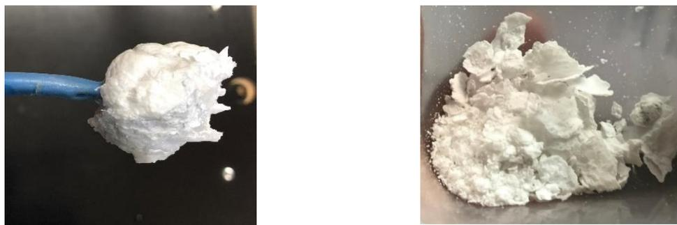
**Fig. 12-** White product observed on ZRP block at the end of anode life testing
