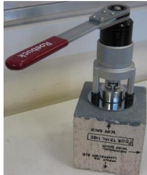
129 **Fig. 1-** Bond strength test setup
