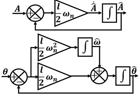
Figure 5: Linearized model of AO-FLL.
