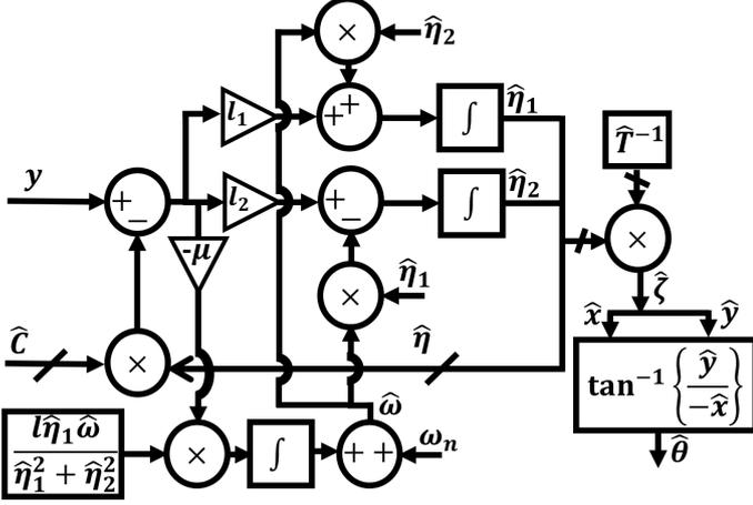
Figure 3: Block diagram of the AO-FLL where matrix multiplication is indicated by  $\rightarrow$ .
