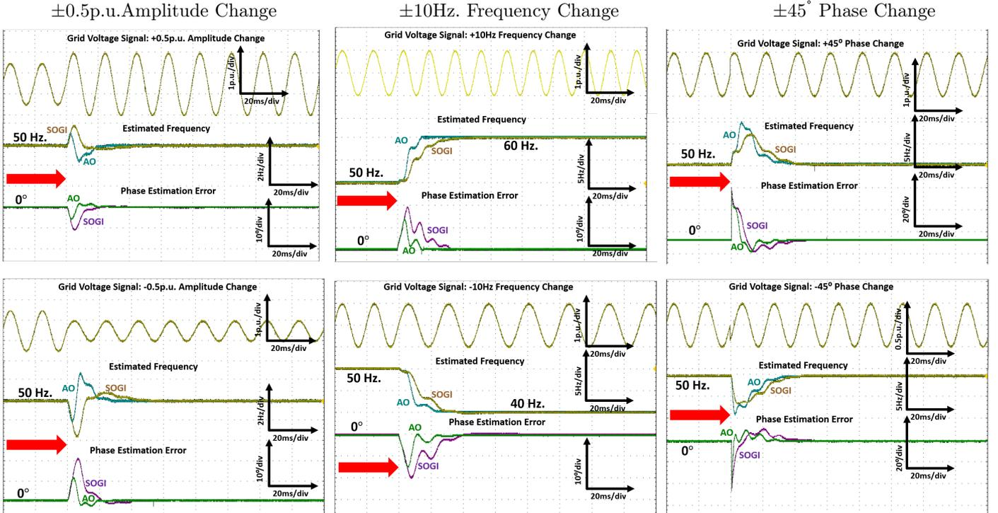
Figure 7: Comparative experimental results for discontinuous jumps in phase, frequency and amplitude.
