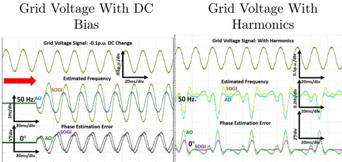
Figure 8: Experimental test results for harmonics and DC bias.
