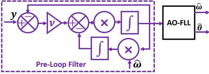
Figure 4: Block Diagram of AO-FLL-WPF.
