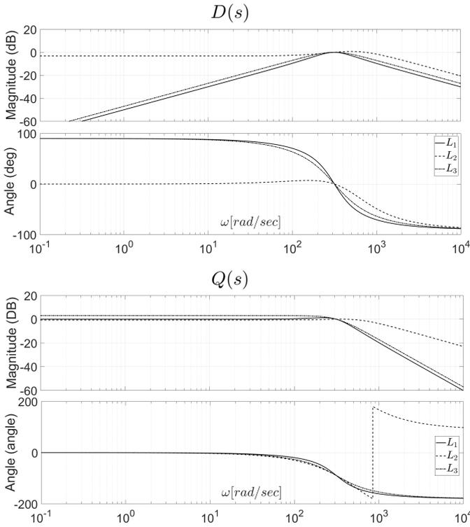
Figure 1: Bode diagrams of the transfer functions (11) and (12) for different observer gains. Transfer functions are obtained by considering closed-loop poles in  $-\omega_n/2 \pm i\sqrt{3}\omega_n/2$ ,  $-1.5\omega_n \pm i\omega_n$  and  $\omega_n/\sqrt{2} \pm i\sqrt{\omega_n}/2$  corresponding to  $L_1 = [0.5; 0.5]$ ,  $L_2 = [0.375; 2.6250]$  and  $L_3 = [1/\sqrt{2}; 1/\sqrt{2}]$  respectively.
