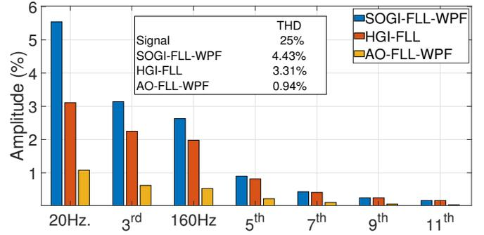
Figure 10: Comparative results of harmonic distortion.
