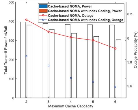
Fig. 2. Power consumption / Outage probability v.s. The cache capacity of users,  $\bar{C}$
